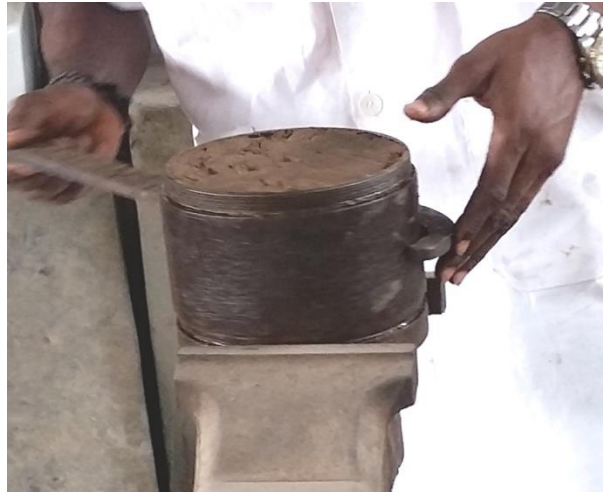
Plate 2. Uncoupling the CBR mould with soil from the collar
