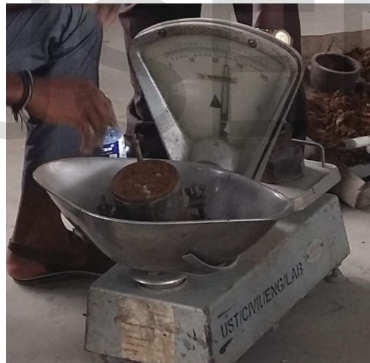
Plate 1. Weighing of compacted soil sample in the mould
